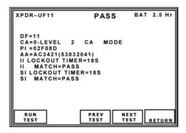
Comprehensive II/SI code and lockout timer test
