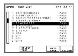
The test list is selected from the auto-test screen. This provides an easy means of selecting any of the individual tests that comprise the auto-test.
